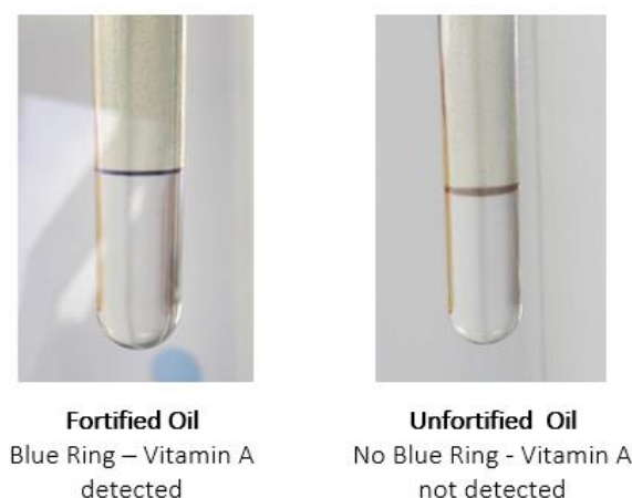
Figure 37: Qualitative Analysis of the Presence of Vitamin A in edible oil using the ring test.
